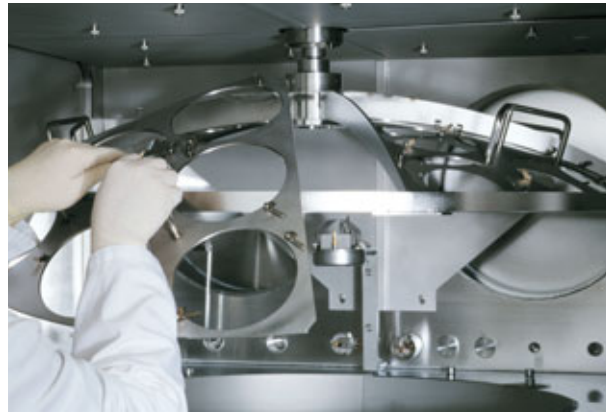
Operator Removing Lift-Off Dome Segment from FC-4400
